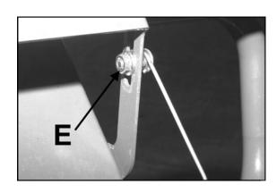
chain tension will reduce chain and bearing life. It can also lead to fatigue failure of the frame.
